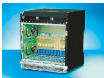
AdvancedTCA® chassis with backplane
