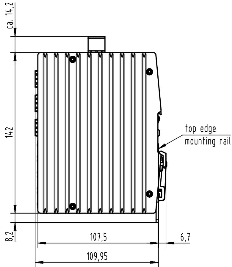
for mounting rail acc. to DIN EN 60715
